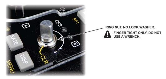
2. Page A4 (Parts List), Front Panel (Top Cover) Hardware (E850532):: Add the following parts:
